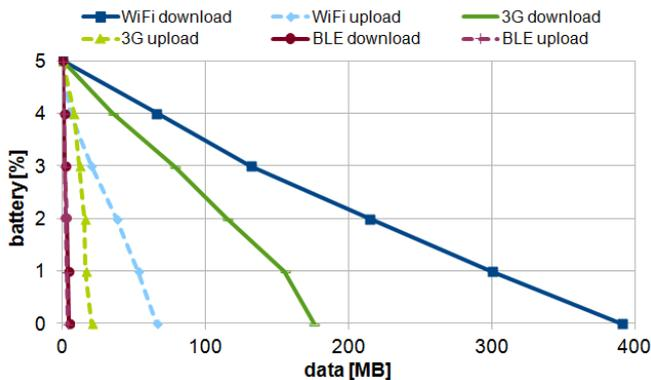
Fig. 1. Amount of data compared to energy consumption
