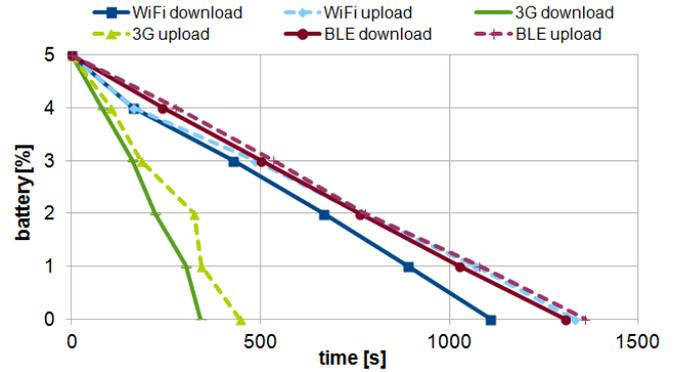
Fig. 2. Amount of elapsed time compared to energy consumption
