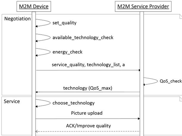
Fig. 3. Process of photo transfer
