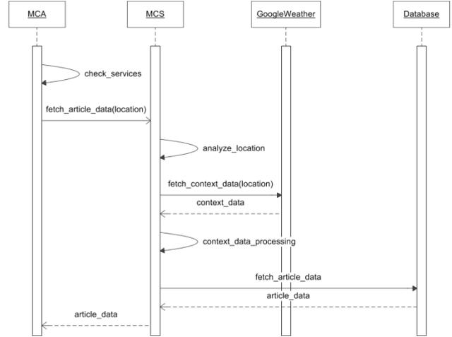
Figure 2. Sequence diagram of receiving recommendations
