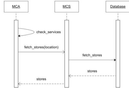
Figure 3. Sequence diagram of receiving store data
